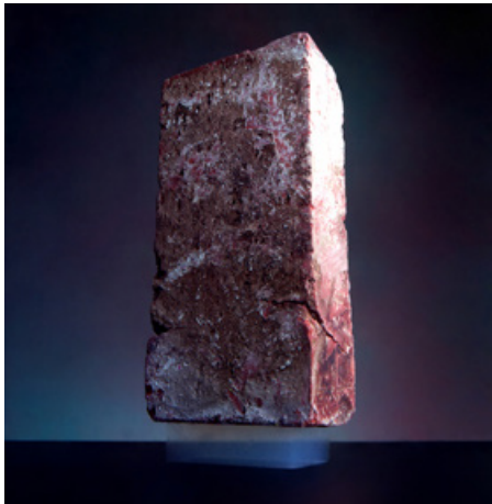
A 2.5 kg stone block is supported by 2 grams aerogel base.
